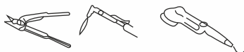
USE ONLY PROPER STEEL SCISSORS. OXYACETYLENE FLAME AND DISC CUTTERS CAUSE SPARK HARMING COIL TO BE ABRADED.
