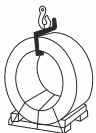
SLING COIL HORIZONTALLY. C-HOOK STEEL IS RECOMMENDED TO HELP BALANCE THE COIL.
